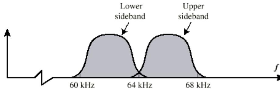
(b) Spectrum of  $s_1(t)$  for  $f_1 = 64$  kHz
