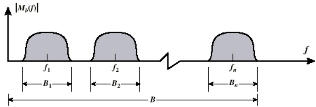
(b) Spectrum of composite baseband modulating signal
