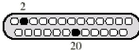
1. DTE A turns on the DTE ready pin (20) to tell its modem it wants to begin a data exchange. While this signal remains asserted, DTE A transmits a phone number via Transmitted Data (pin 2) for modem A to dial.
