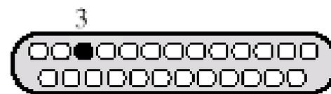
6. Modem B reconverts the signal to digital form and sends it to DTE B via the Received Data pin (3).
