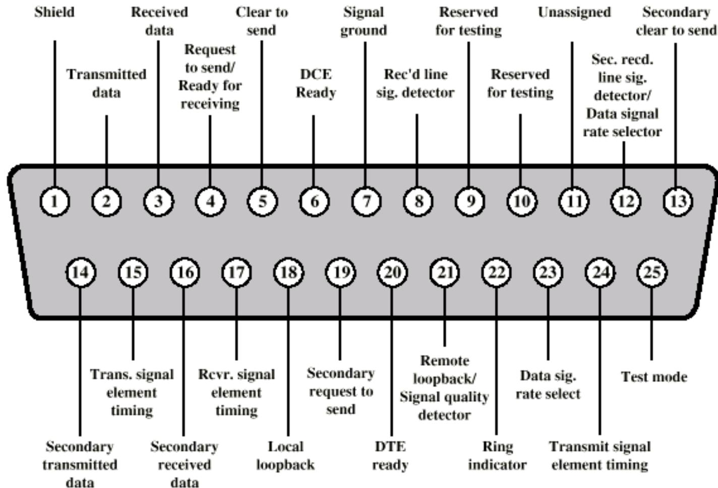
Figure 6.5 Pin Assignments for V.24/EIA-232 (DTE Connector Face)
