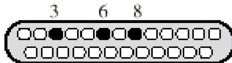
3. When modem A detects a carrier signal, it alerts DTE A via pin 8. The modem also tells the DTE that a circuit has been established (pin 6). If the modem has been so programmed, it will also send an "on line" message to the DTE's screen via the Received Data pin (3).
