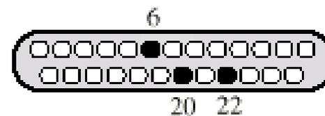
2. When modem B alerts its DTE to the incoming call via the Ring Indicator pin (22), DTE B turns on its DTE Ready pin (20). Modem B then generates a carrier signal, to be used in the exchange, and turns on pin 6, to show its readiness to receive data.
