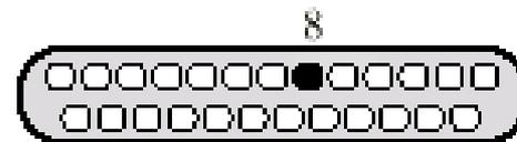
4. Modem A then generates its own carrier signal to modem B, which reports it via pin 8.
