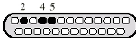
5. When it wishes to send data, DTE A activates Request to Send (pin 4). Modem A responds with Clear to Send (pin 5). DTE A sends data (pulses representing 1s and 0s) to modem A via the Transmitted Data pin (2). Modem A modulates the pulses to send the data over its analog carrier signal.
